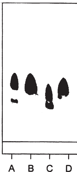
Figure 3. TLC chromatogram of MPEGs. Silica gel (Merck 60 F 254 ): eluent: CHCl 3 - CH 3 OH (10:1.5). MPEG 2000: (a) commercial (Table 1, No. 3), (b) after chromatography (Table 1, No. 5); MPEG 5000: (c) commercial (Table 1, No. 8), (d) after chromatography (Table 2, No. 9).
